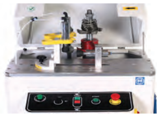
Dikey 1 yatay mengene sistemi 2 vertical 1 horizontal vise system
