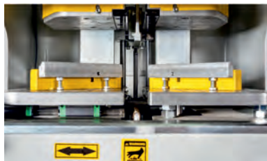
Lineer kızak sistemli hareketli tablo Moving table with linear guide system
